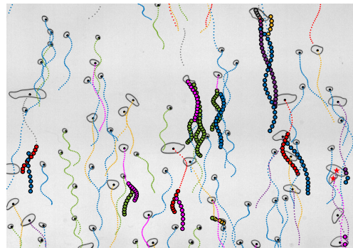
Figure 1: Snapshot of the bubble swarm along with the positions of the bubbles provided by the BTA for previous time steps. Trajectories of bubbles are plotted as dots, colored according to their sizes. Data prior to collisions is highlighted with larger symbols. A collision event is pointed out by red stars.
